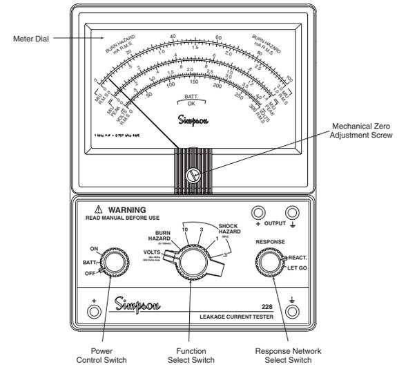
Figure 2. Controls and Functions
